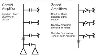
Because all EST3 zoned amplifiers have an integrated backup 1000 Hz temporal tone generator, the locally-generated alarm tones notify occupants of a hazard – even with the primary riser out of commission. The backup tone also operates if the ASU or the audio distribution system fails. To further enhance system survivability, a single standby amplifier can backup any zoned amplifier in the same cabinet.
